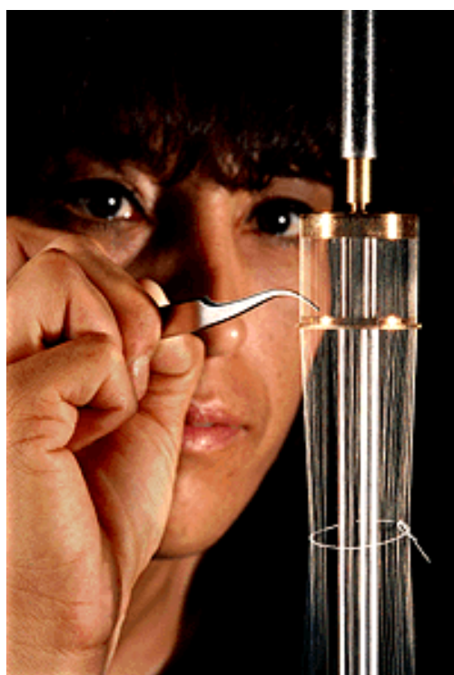
Figure 5-5. A Sandia technician builds an array of wires, each 1/10 th the width of a human hair, that form a target for the Z accelerator.
