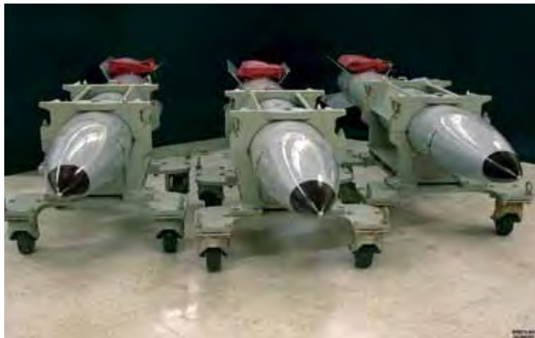
Figure 2-2. B61 bombs represent some of the oldest designs in the active nuclear weapons stockpile. Recent alterations continue the process of extending service lifetime by refurbishing spin rocket motors and some canned sub-assemblies.
